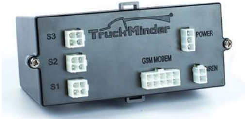
Image 2.1 – Main Control Unit
